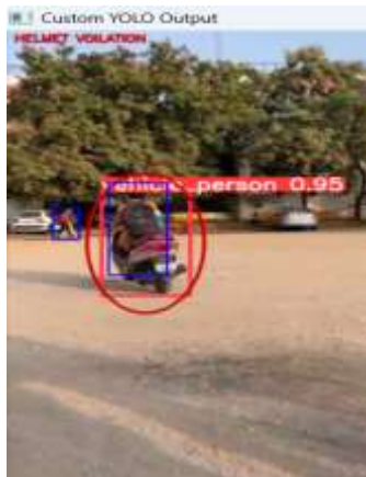
YOLO Output Image (Detection of vehicle_ person, motorcycle, helmet)
